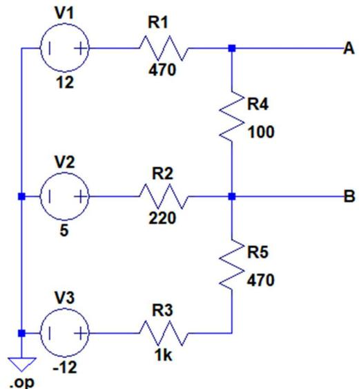
Figure 4. Circuit used in a test of Thevenin's theorem.
