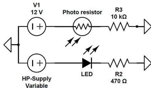
Figure 6. A light emitting diode exciting a photoresistor.
