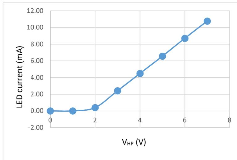
Figure 7. Current through the LED plotted versus  $V_{HP}$ .
