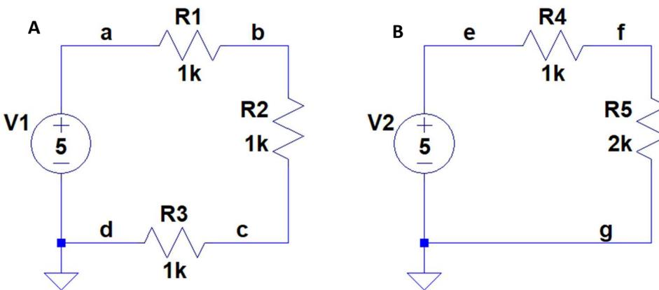
Figure 1 (A) Three series resistor circuit, (B) two series resistor circuit.
