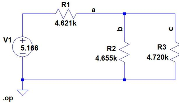
Figure 2. The circuit used to confirm the combination of parallel resistors and KCL.
