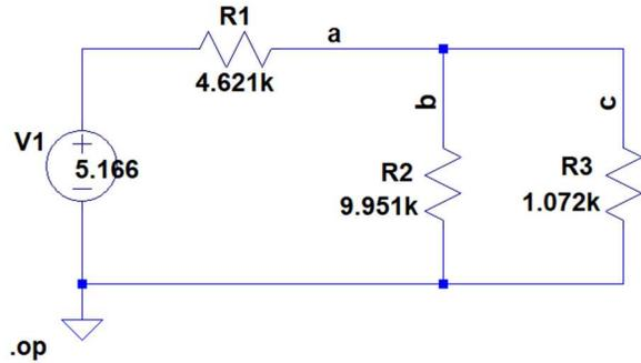
Figure 3. The circuit of Fig. 2 modified with a nominally 10k and 1k resistor in parallel.
