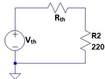
Figure 5. Thevenin's equivalent circuit.
